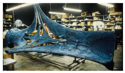
over a simple frameworks of angle iron. By attaching old fashioned garter snaps at various strategic places we could pull the spandex into the shape required and achieve the smooth aerodynamic design Sid had envisioned. That done we saturated the spandex with epoxy resin
