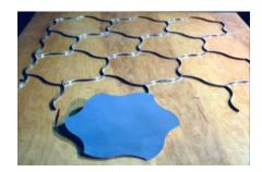
We finally settled on a pattern like this, which is a hexagon with a sine wave replacing the straight edges. These "tiles" produced a homogenous surface which worked very well.
