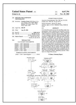
The gist of Reverse Bluescreen is that we can exploit motion control technique to acquire a separate matte record. We simply coat the subject with an invisible phosphor that only glows under blacklight. By making multiple passes sequentially under white light and black light, we can obtain our mattes much as with Sodium Vapour. But the big advantage here is the elimination of "spill" light on the subject. But, of course we couldn't use this solution for live action.
