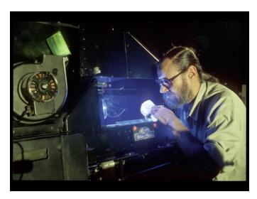
Blue-Max, of course, was somewhat more sophisticated than that. We use a short arc Mercury vapor light and add dichroic interference filters to isolate the 436 nm Mercury line, and we provided quite a deft way to "dim" a discharge light.
